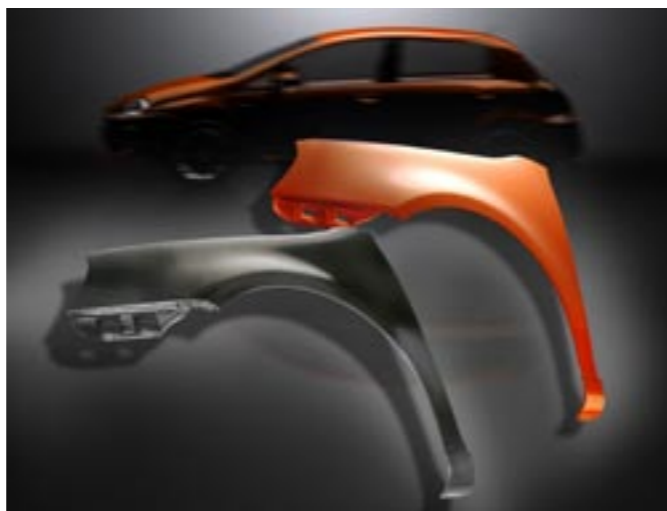
Ultramid TOP 3000 can be coated on-line with the rest of the metal car body.
